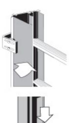
20.Lift and place ladder section on top of base section rotating to engage mounting blocks on brackets.
