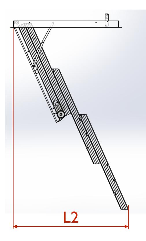
NOTE: The L2 values in the table below are for information only. Depending of the final Stairway configuration the value of L2 can be decreased or increased for any ceiling height.
