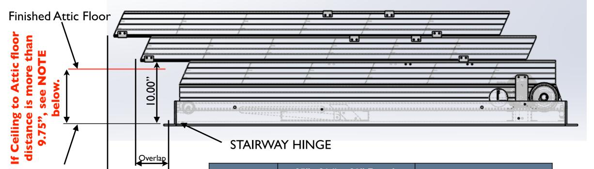
Above picture is generic. It shows 2 sliding sections of 6 steps each whereas the Stairway might have 3 sliding sections of 5 to 9 steps each. The resulting overlap of each section will therefore vary (see NOTE below).
