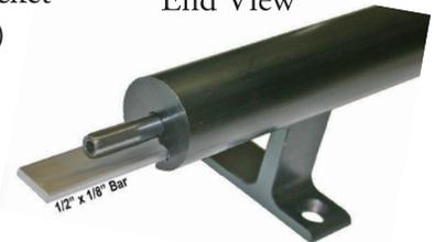
(C) Tap the end of the rail with a 1/4" x 20 tap (not supplied) to screw in the end stop finial (done before installation of rail). Install end stop with screw provided.
