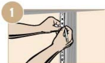
Mark drill hole locations. For safety, space cables no more than 3 inches apart and have a post or vertical spacer at least every 3 feet. See [this page](#) for frame requirements.
