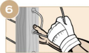
Hold the Quick-Connect® SS fitting with one hand and pull the cable tight with the other. The Quick-Connect® SS automatically locks when you release the cable.
