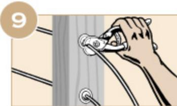
Using cable cutters or an electric grinder with cut-off disk, trim the excess cable from behind the Quick-Connect® SS fittings. Grind flush the exposed cable ends with a grinding disk.
